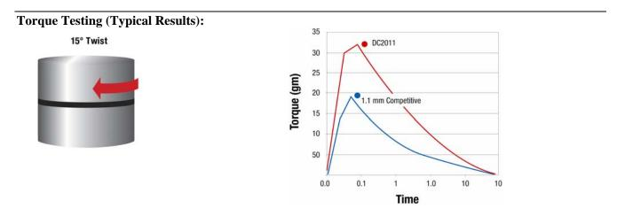
3M Series DC2000 tape demonstrates higher resistance to twisting forces (torque) compared to typical competitive tapes.
