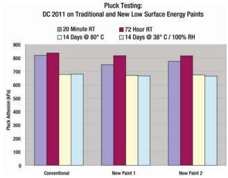
Maintains pluck adhesion on new low surface energy and scratch- and mar-resistant paint systems in addition to conventional paint systems.
