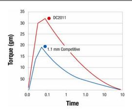
3M Series DC2000 tape demonstrates higher resistance to twisting forces (torque) compared to typical competitive tapes.
